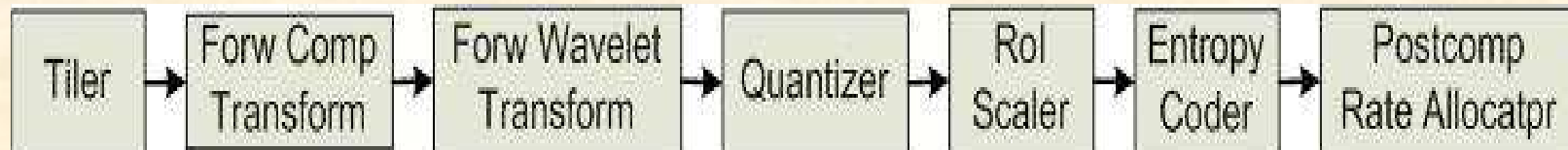
(a). Diagram Blok Proses Encoding JJ2000
