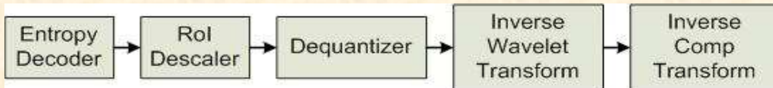
(b). Diagram Blok Proses Decoding JJ2000
